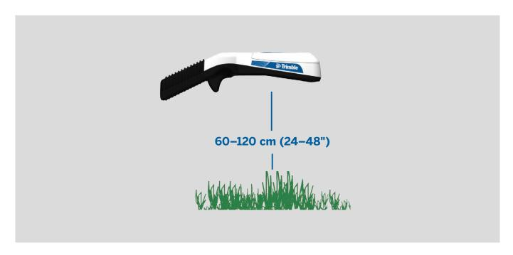
To ensure the accuracy of your readings, hold the sensor 60-120 cm (24"-48") above the crop when the trigger is pulled.
