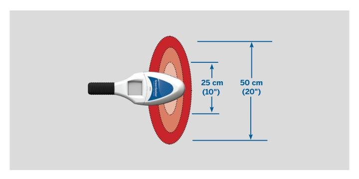
The sensor's field of view is an oval; the field of view widens as the height of the sensor above the ground increases.
