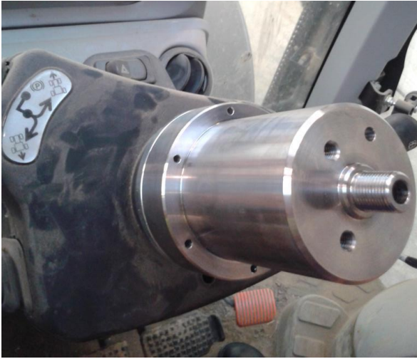
Figure 17. Installation of the RMT Bush
