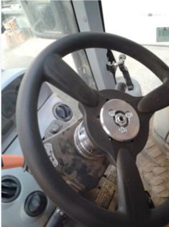
Figure 24. Manual steering with the Trimble Steering Wheel disconnected
