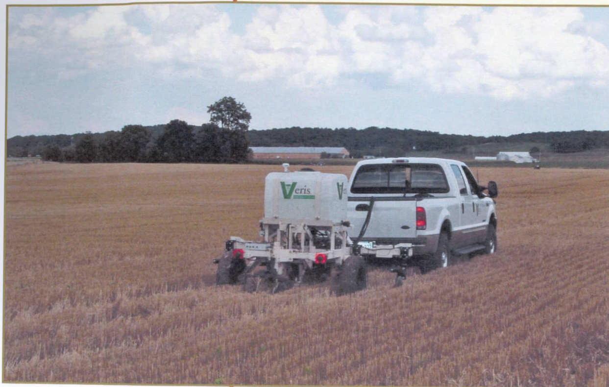
Fig. 6. Veris Mobile Sensor Platform with on-the-go pH measuring.
